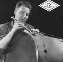
REAL REGULATION of new G-E thermocouple assembly on jet engine comes after its manufacturing steps.
